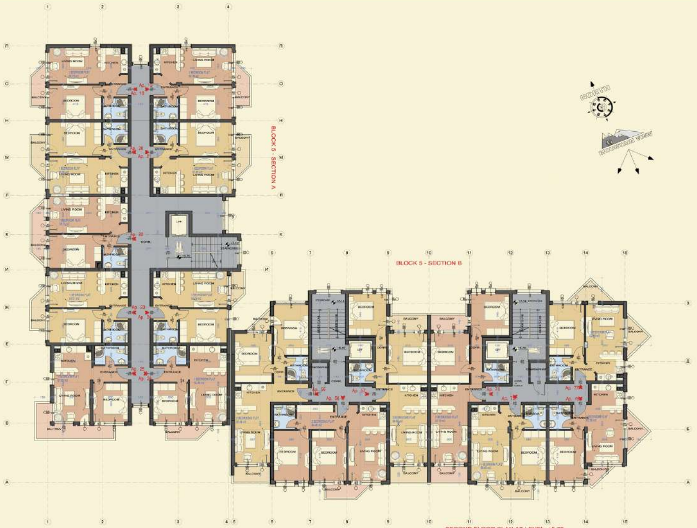
SECOND FLOOR PLAN AT LEVEL +5.70 SECTION 1 - AREA - 507.85 m 2 SECTION B - AREA - 494.65m 2
