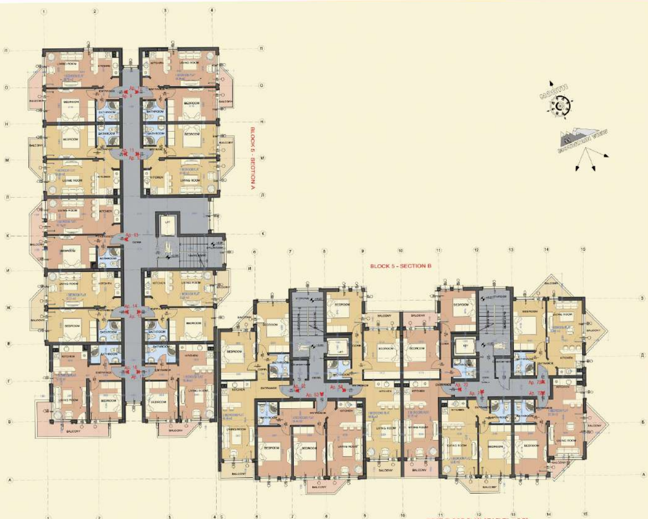
FIRST FLOOR PLAN AT LEVEL +2.95 SECTION 1 - AREA - 507.85 m2 SECTION B - AREA - 494.65m2
